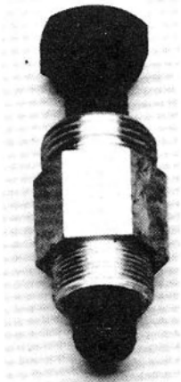
MAGNETO FLYWHEEL PULLER (Bosch - C.E.V. - Dansi)
